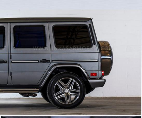
While it looks essentially stock – even retaining the factory side exhaust – the INKAS® G63 is fully armored, with a reinforced roof, doors, glass, quarter panels, firewall and pillars.
