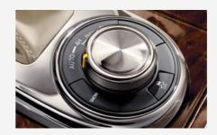
HOLD THE ROAD As driving conditions change, the All-Mode™ AWD system is ready. Set it to AUTO and the system continually adjusts the amount of power distributed between the front and rear wheels for enhanced control. If any wheel should slip, the Traction Control System helps redirect power toward the wheels with traction. The system also has settings for 2WD, 4WD High and 4WD Low for times when you need high traction, like in loose terrain or on steep inclines.
